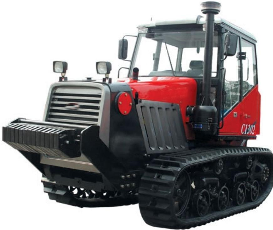
Crawler tractor-C1302 belongs to the 100-130HP crawler tractor section. This product is primarily designed for agricultural jobs. In addition, it can also be used for bulldozing operations in common earth works. This tractor is equipped with LR6A3Z-22 diesel engine, which is reliable and powerful. Dozer blade is available to suit your specific requirements. The track shoe width is 390mm, and the wheelbase is 2774mm.
