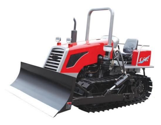
Crawler tractor-C502 is a product of 40-60HP crawler tractor series. It is equipped with a dozer blade and B2-22 diesel engine. The track width is 310mm, the wheelbase is 1600mm, and the ground pressure is 34.58 kPa. Features:
