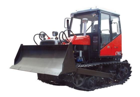
Crawler tractor C902-2 is a primary product of 70-90HP crawler tractors. This type of tractor is based on C902 caterpillar tractor; however, it is more suitable for bulldozing operations due to its adoption of(4F+2R)sliding gear transmission. Quality built and economically priced, our crawler tractor is widely used for irrigation, pond renovation, small town construction and so on.
