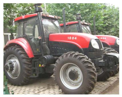
The tractor BN-X1604, 160HP, 4WD is developed on the basis of the Italian wheeled tractor chassis technology, adopting the British technology-based 6-cylinder turbocharged engine, which is featured with low specific fuel consumption and better power economic efficiency. The tractor has multiple gears, a wide speed range, and a large capacity of fuel tank, ensuring long-time operations with a single fueling. Besides, it is flexible in steering and easy to operate.
