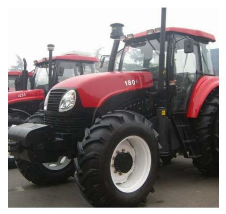
The Tractor BN-X1804, 180HP, 4WD is developed on the basis of the Italian wheeled tractor chassis technology, adopting the British technology-based 6-cylinder turbocharged engine, which is featured with specific low fuel consumption and better power economic efficiency. The tractor has multiple gears, a wide speed scope, and a large capacity of fuel tank, ensuring long-time operations with a single fueling. Besides, it is flexible in steering and easy to operate.
